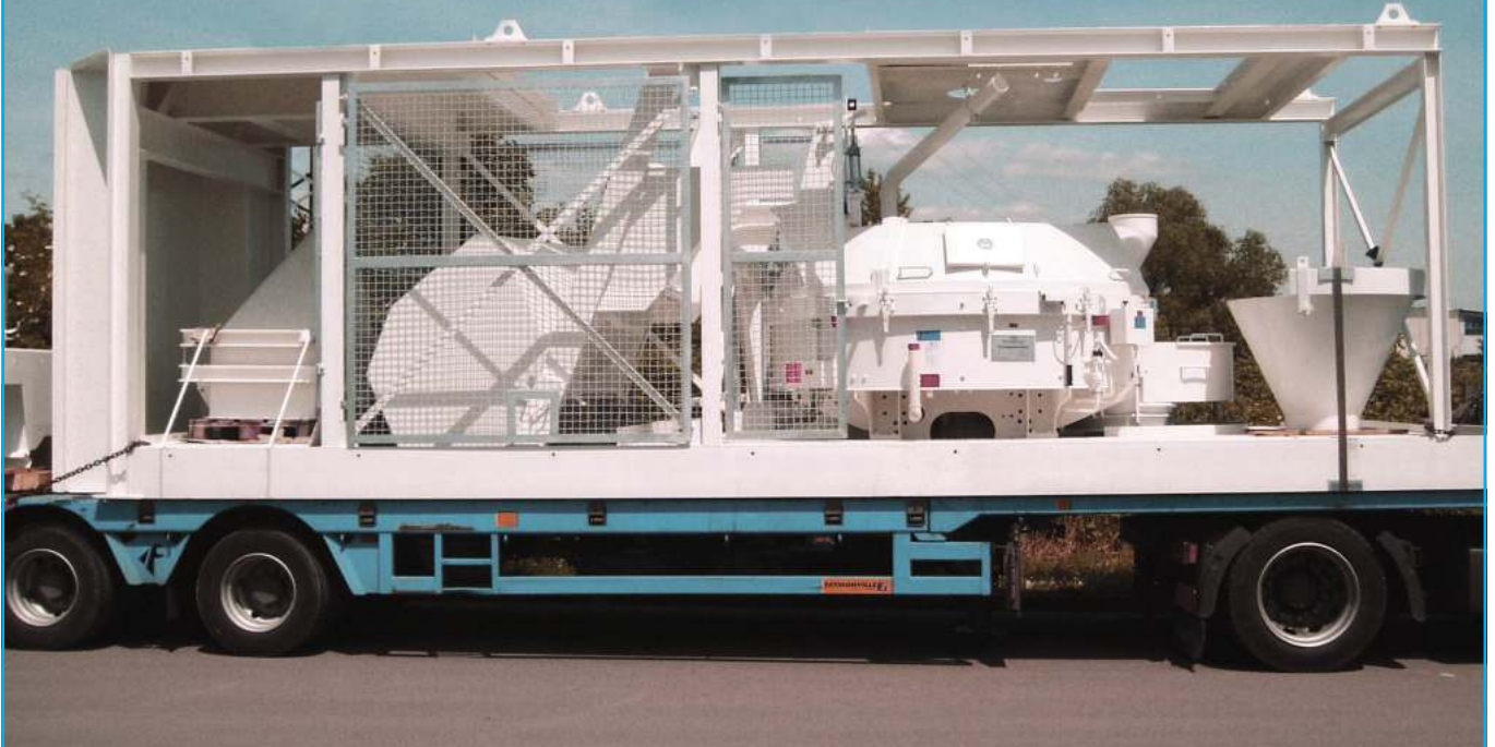
Transport MIXOMAT THZ 1500 B - S 5 Sternanlage • Transport MIXOMAT THZ 1500 B - S 5 scraper system
