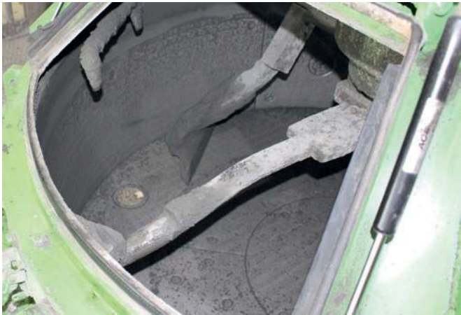
Moisture measuring sensor in the base of the mixer
