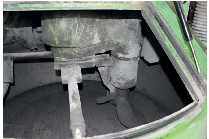
The specially designed scraper on the shaft is now installed as standard in all turbine mixers.
