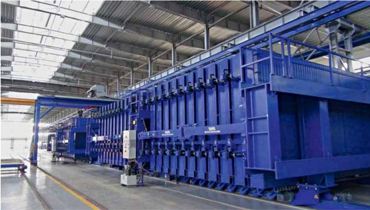
Up to 1,500 m<sup>2</sup> of precast concrete elements are manufactured per day on three battery molds of the latest generation
