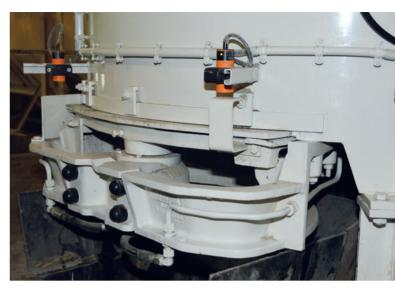
Teka discharge gates are operated by a powerful hydraulic rotary cylinder. If needed, multiple proximity switches can be added to allow for partial openings of the gate.
