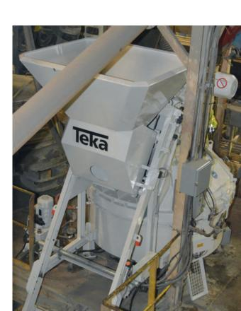
The Teka Skip Hoist has a bottom-discharge bucket, and travels on the 60° angle track, quickly delivering batch materials to the mixer, which is over 25′ above the plant floor.
