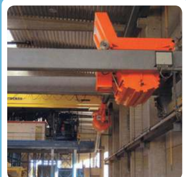
Rollover bucket and concrete distributor
