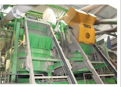
Teka installed two skip hoists (500 litres) in a bottom discharge design to complement the two new facing concrete mixers.
