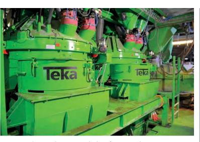
The two Teka THT E-1-III high performance turbine mixers for high-quality facing concretes.
