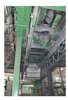
Like the core concrete mixers, the new high performance turbine mixers discharge directly into one of the two flying buckets.
