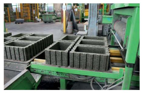
Two concrete block lines run at the Kretz site, on which virtually the complete product range from the areas of concrete paving stones and slabs as well as numerous pumice products are manufactured.
