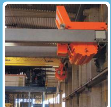
Rollover bucket and concrete distributor
