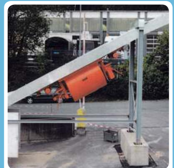
Rollover bucket in a 32° inclination = 60%
