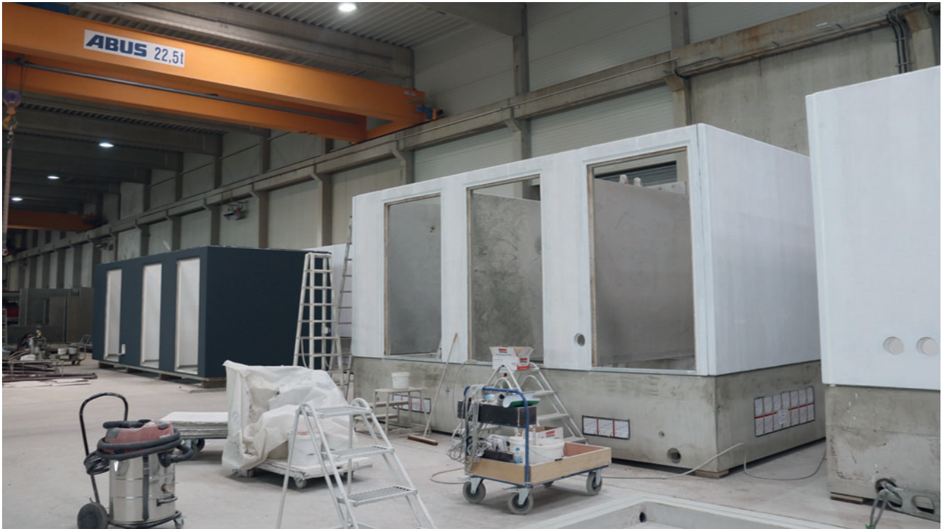
On average, 150 man-hours go into a transformer station until it is ready for dispatch.
