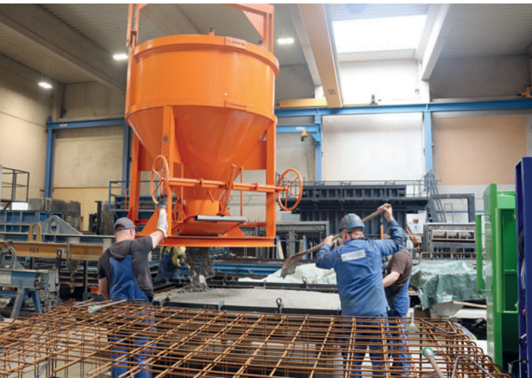
The concrete is distributed in the production area by means of buckets and overhead crane in the main hall. The buckets are transported to the adjacent hall by a Muli-Trans electric platform truck
