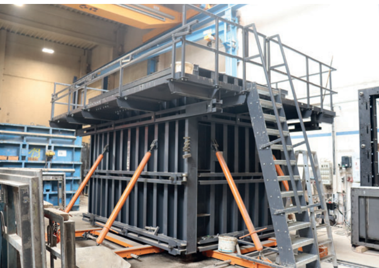
A 3D formwork from Ratec for the production of transformer station elements is also one of the latest investments at the Arnstadt site.
