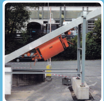
Rollover bucket in a 32° inclination = 60%
