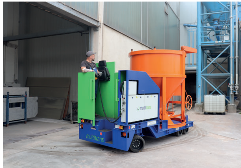
The concrete is distributed in the production area by means of buckets and overhead crane in the main hall. The buckets are transported to the adjacent hall by a Muli-Trans electric platform truck
