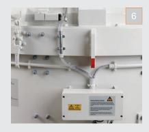
**6** | Electrical components are completely pre-wired to an electrical junction box.
