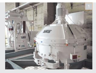
**1** | The THT mixer is ideally suited for face-mix, fiber-, foam-, self-compacting-, color-, ultra-high-strength concrete, etc. This mixer type is also optimally suited for the absolute smallest batch sizes (partial loadings), and therefore extremely variable in its use.
