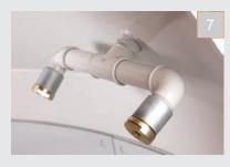
**7** | Production water is sprayed into the mixer through multiple nozzles.
