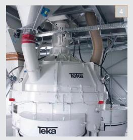
4 The mixer hood design has several large areas for material inlets. Cleaning/access doors can be installed in various locations, and are built with quick-release latches and gas-pressure pistons to keep them open. Electronic safety switches stop mixer operation when access doors are opened.
