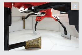
2 Mixer models THT 250 - 1125 have one mixing turbine. THT 1500 - 2250 models can be fitted with either one or two mixing turbines, and the THT 3000 can have either one, two or three mixing turbines.
