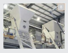
8 All TEKA mixers can be outfitted with a Skip Hoist to charge the mixer with batch materials. TEKA offers tilting skip hoists for very steep angles (90°) of inclination, or the standard 60° nontilting bottom-discharge type.
