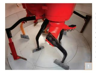
1 | The efficient and aggressive mixing action of batch materials results in maximum homogenization in the shortest possible cycle times. Even the most demanding batch designs are thoroughly mixed, due to the effective design and rotation of the mixing arms and paddles.
