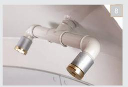
8 | Production water is sprayed into the mixer through multiple nozzles.
