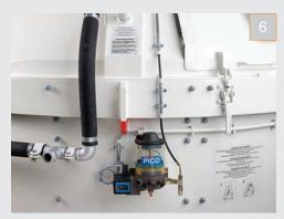
6 | TPZ mixers have low maintenance factors, and require gearbox oil changes only every 2500 hours. Central grease lubrication (except for rotating mixing stars) is standard. An optional motor-driven automatic grease lubrication pump is available.
