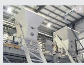
9 All TEKA mixers can be outfitted with a Skip Hoist to charge the mixer with batch materials. TEKA offers tilting skip hoists for very steep angles
