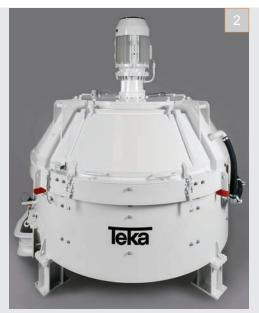
2 | TPZ mixers have a low overall height due to the externally mounted discharge gate, and offer easy access to the inside of the mixer.
