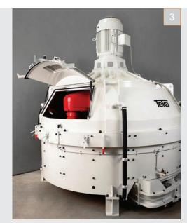
3 | The robust and compact design of the drive line uses only one motor for high efficiency. Hydraulic Turbo Couplings are standard on the TPZ 1500 and larger models. As an option, a frequency converter can be installed on all TEKA mixers, to optimally adjust the speed of the mixing arms.
