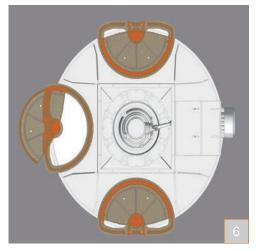
6 | Models THZ 250 to THZ 750 can be built with up to 4 discharge gates. Models 1125G to THZ 6000 can have up to 3 discharge gates. Sample gates are also available.
