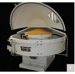
7 | A protective mixer hood encloses the mixer pan. A built-in seal makes it near dustproof. Large, hinged segments with variable openings are possible, raised and lowered by a manual- or motorized cable winch. With no components located above the mixer hood, there are no obstructions to impede the arrangement of cleaning segments,
