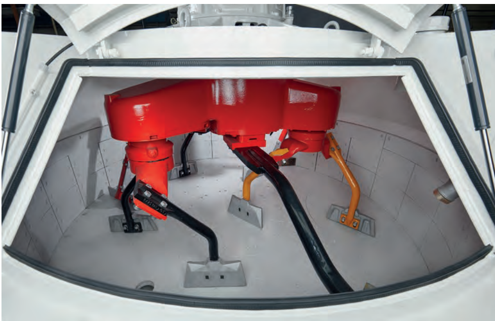
Inside view of the TPZ planetary mixer.
