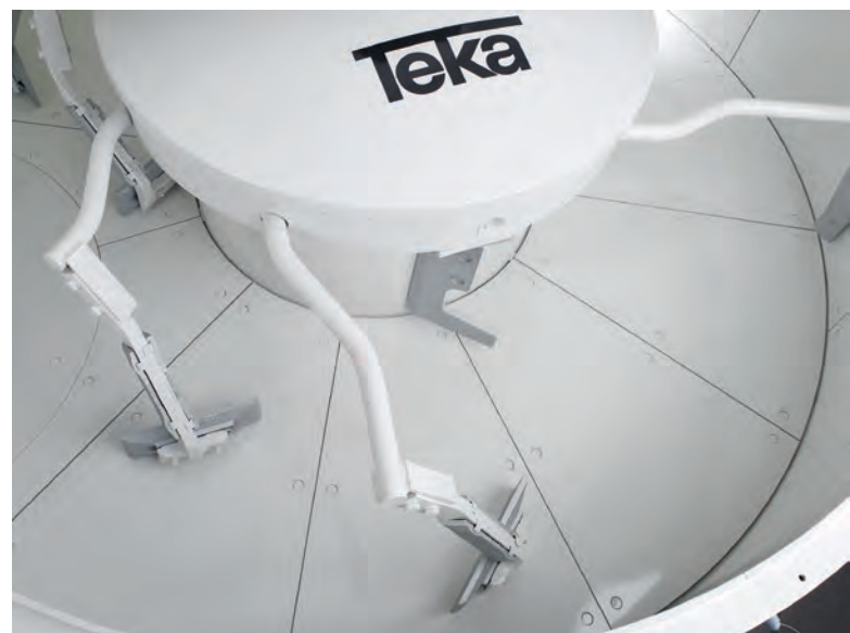
The Teka THZ pan mixer features spring-loaded mixing arms that are adjustable to compensate for wear.
